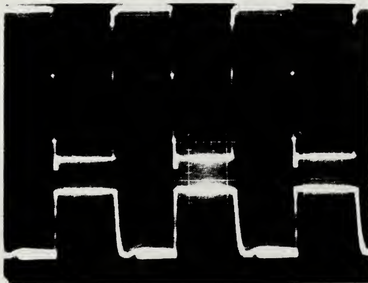
Figure 3.6 Top Trace, 150 KHz Transmitted Signal Bottom, Received Signal Through 10898 m Fiber (Top 1v/Div, Bottom 10mv/Div @ 2 usec/Div)
